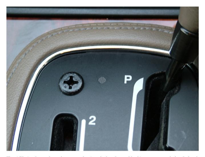
The LED is shown here between the interlock release blanking screw and the P (park position)
