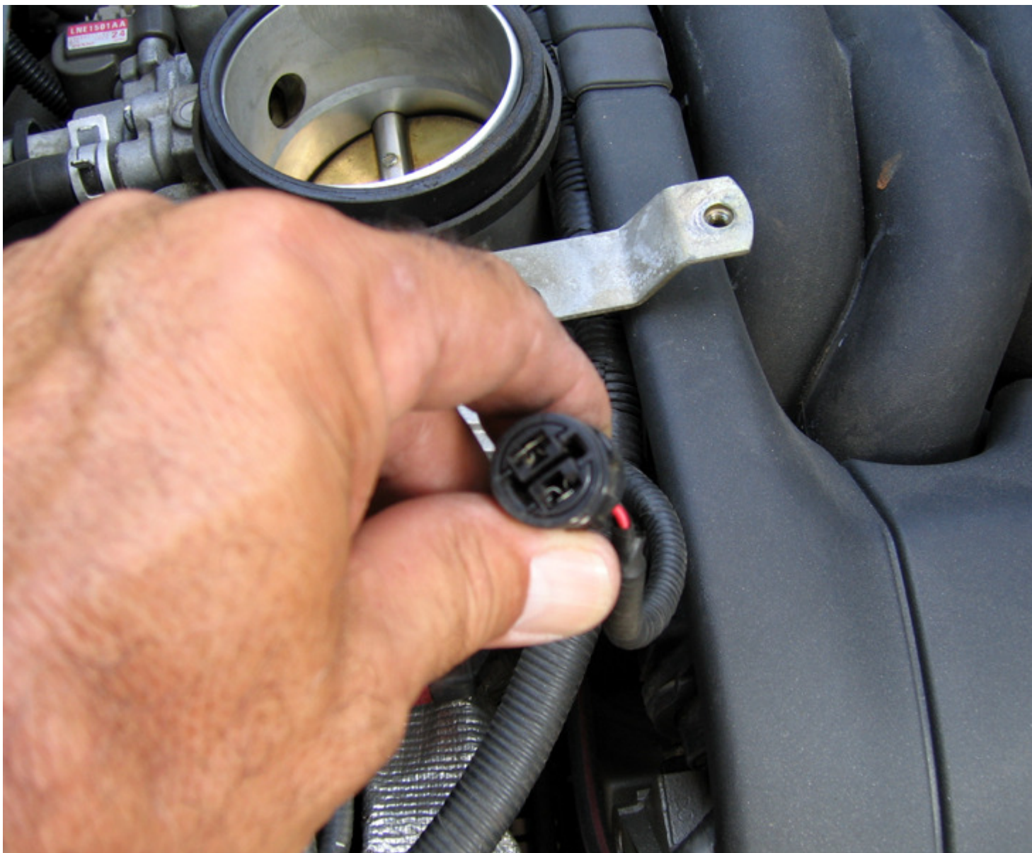
Found that the plug stays were broken
