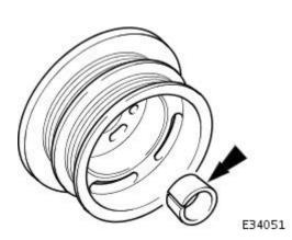
11. Remove the internal O-ring seal.
