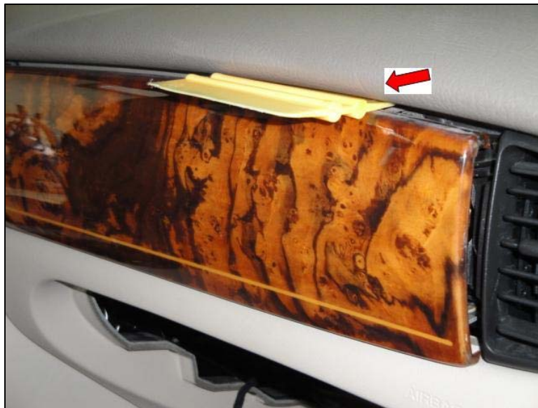
Detachment of the wood trim panel using a plastic tool
