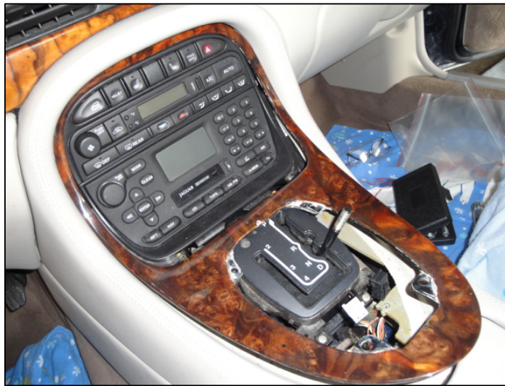
Console wood finish “ski slope” trim detached from the console.
