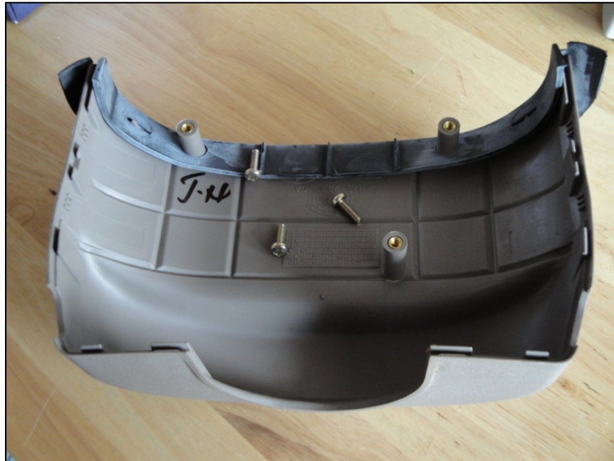
The underside of the upper steering cowl, showing its three mounting bolts
