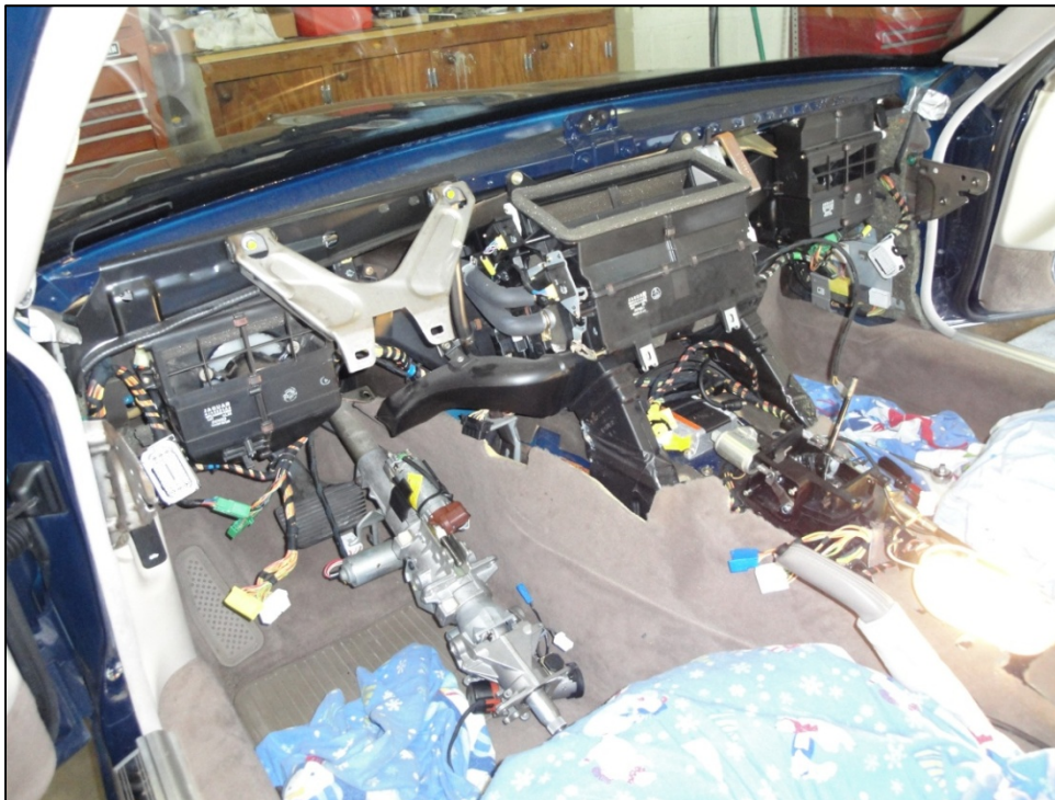
Driver's side view after fascia board removal, revealing the Evaporator/Heater Box
