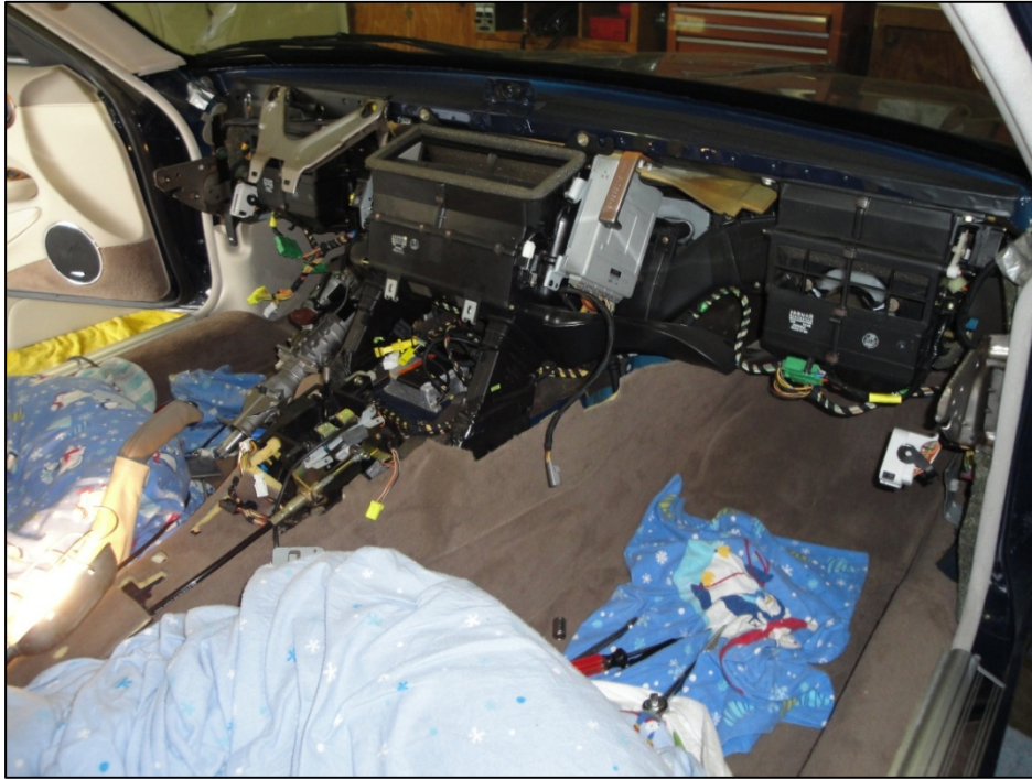
Passenger's side view after fascia board removal, revealing the Evaporator/Heater Box
