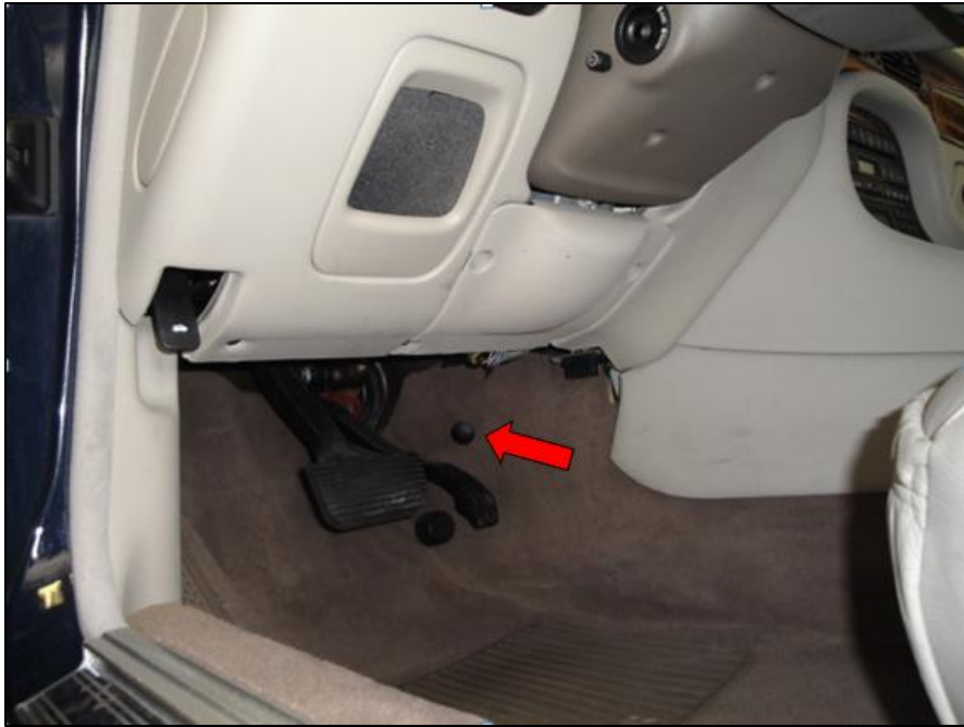
Location of fir tree connector holding the carpet to the driver's side tunnel.
