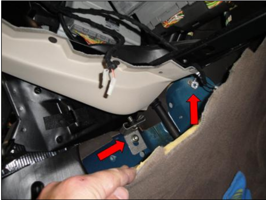
Locations of grounding wire stud and mounting bracket on the passenger's side.
