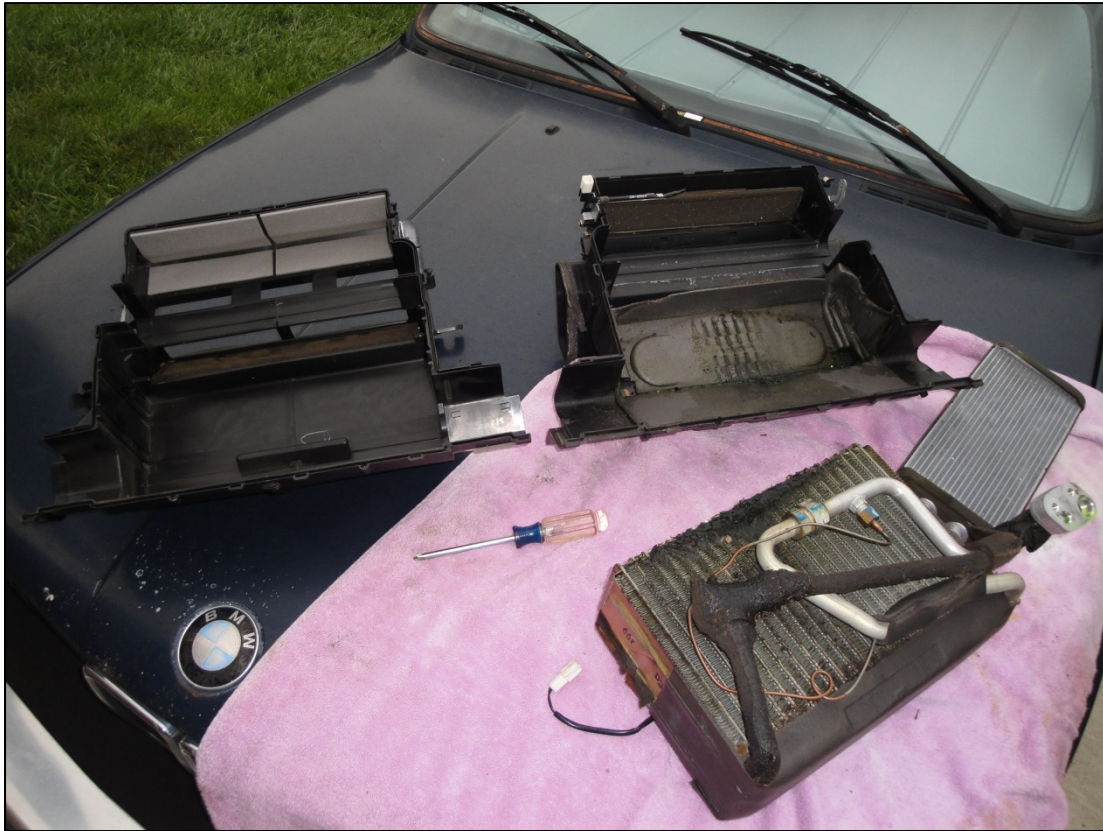
Heater/evaporator box separated, showing its two halves as well as the heater and evaporator cores removed.
