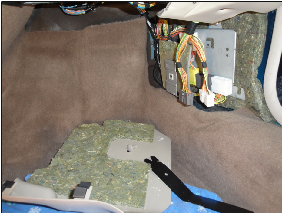
Passenger side foot well panel removed, showing fir tree connector, electrical connectors, and metal clips.
