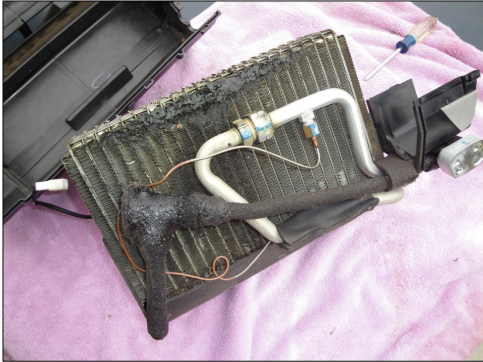
Failed evaporator core showing buildup of oily debris
