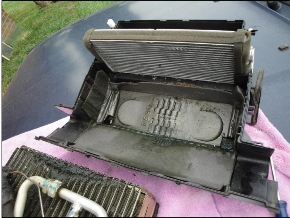
Dirty evaporator box, with heater core still in place, contaminated with debris and refrigerant oil.
