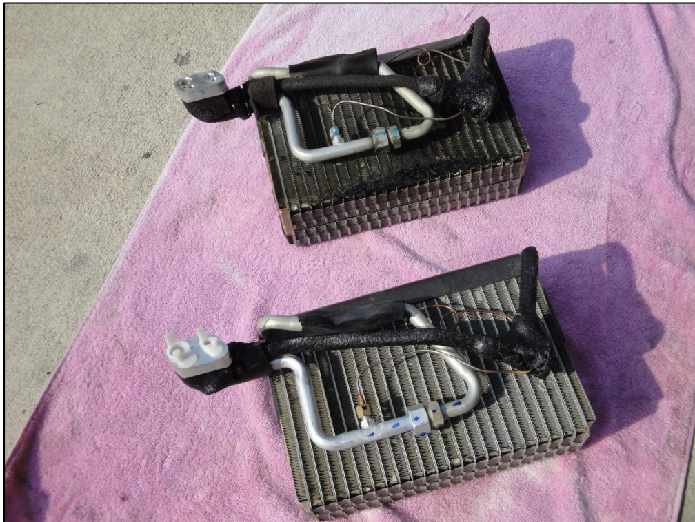
The defective evaporator core alongside its new replacement
