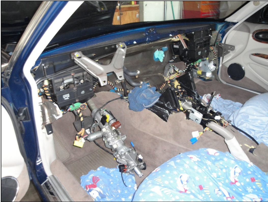
Driver's side view after removal of the heater/evaporator box
