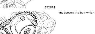
**15.** Loosen the bolt which secures the sprocket to the camshaft.
