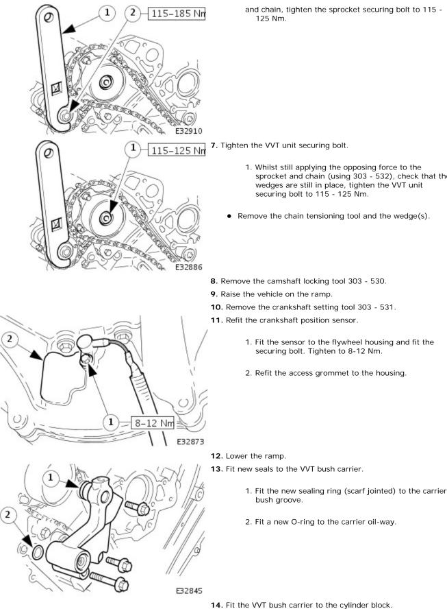
and chain, tighten the sprocket securing bolt to 115 -
