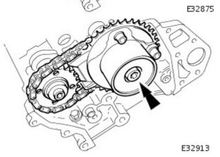
**16.** Loosen the bolt which secures VVT unit to the camshaft.
