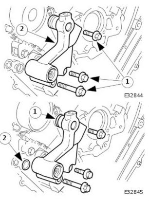
2. Release the carrier from the two ring dowels and remove it.
