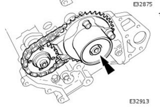
**16.** Loosen the bolt which secures VVT unit to the camshaft.
