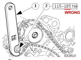
and chain, tighten the sprocket securing bolt to 115 - 125 Nm.
