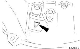
**11.** Fit the crankshaft setting peg 303 - 531 to the crankshaft position sensor location.
