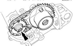
**15.** Loosen the bolt which secures the sprocket to the camshaft.
