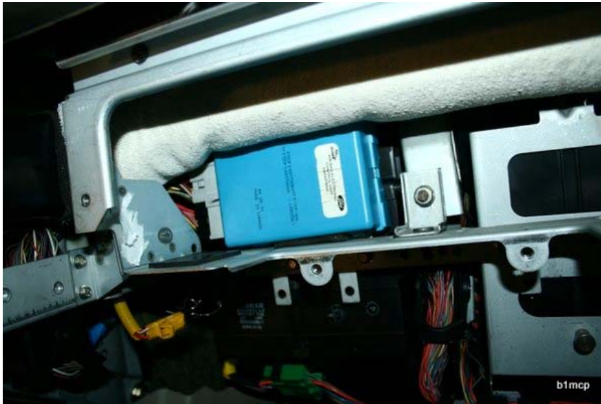
Location of the Air Bag ECU. This sits directly behind the Passenger Air Bag (which has been removed in this picture)
