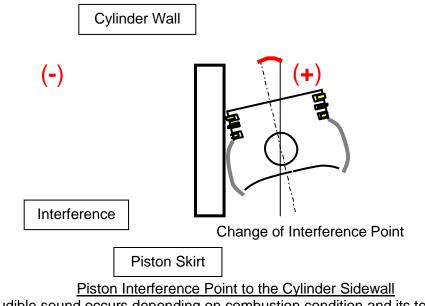
The audible sound occurs depending on combustion condition and its temperature.
