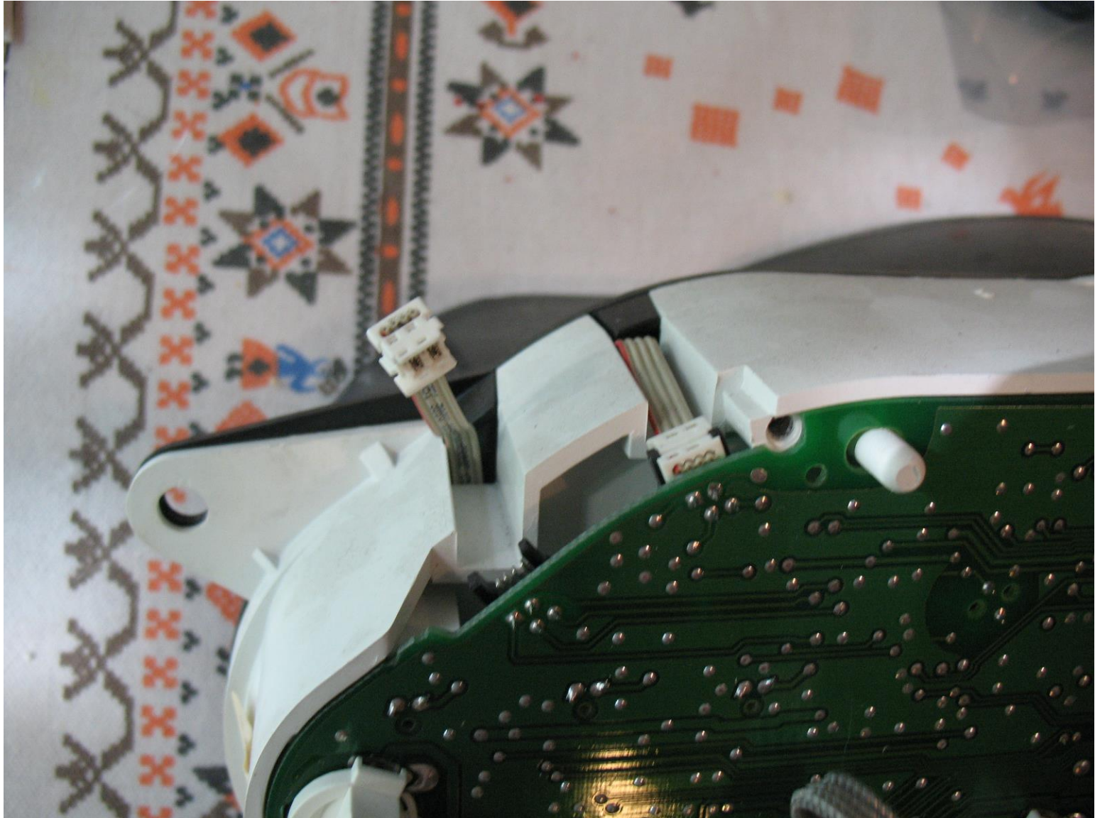
Ribbon Connector disconnected from the main circuit board
