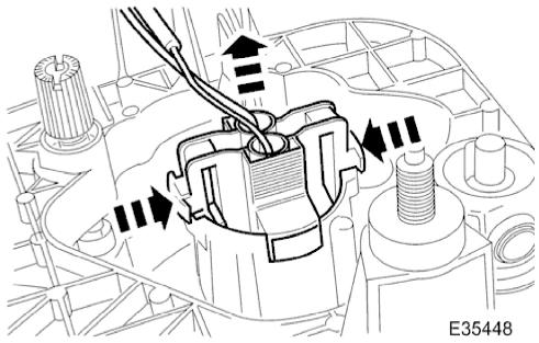
2. Release bulb holder securing tangs and position holder for access.
