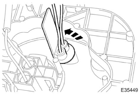
3. Install pilot bulb holder in headlamp unit and rotate 1/4 turn to secure.
