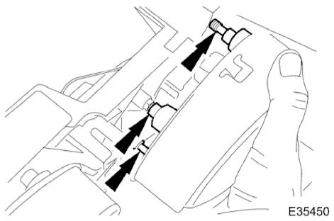
5. Release headlamp unit adjusting screws and pivot.
