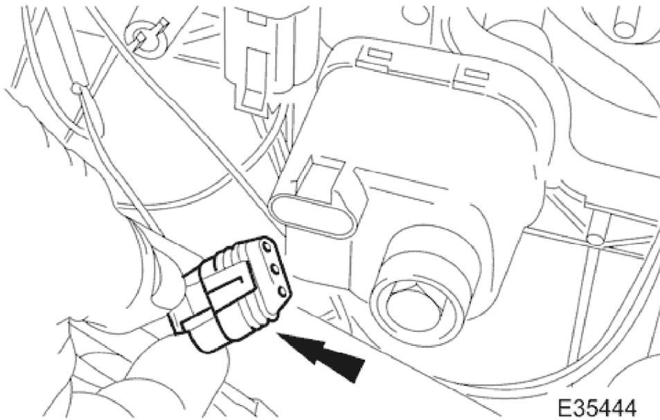
4. Connect headlamp levelling actuator harness connector if fitted.
