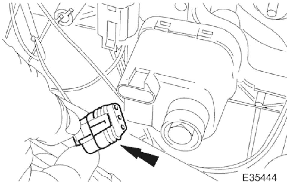
4. Disconnect headlamp levelling actuator if fitted.
