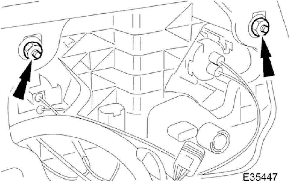
1. Position headlamp assembly on body and install upper nuts.
