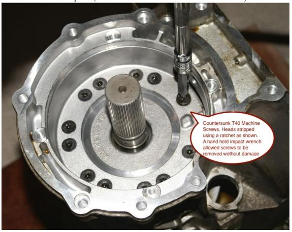
I initially tried to remove them using only a 3/8" ratchet but found I damaged the Torx head on the 1<sup>st</sup> two I tried, stripping one so badly I had to drill it out. I then reverted to a hand held impact wrench and found that all screws released after a couple of hard smacks & could then be removed using the ratchet. I replaced all the retaining screws with Hex Socket units sourced locally at a cost of @ \$5.
