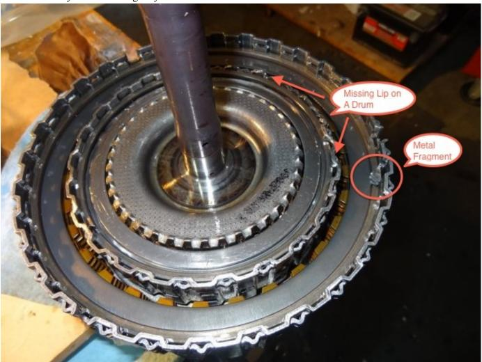
A section of the lip of the drum approximately 3" long and ¼ "wide had broken off the top of the drum at the capture point for the snap ring which holds the clutch pack in place. While the snap ring was still in place, the missing lip allowed fluid to leak by preventing the clutch from operating. This appears to be the
