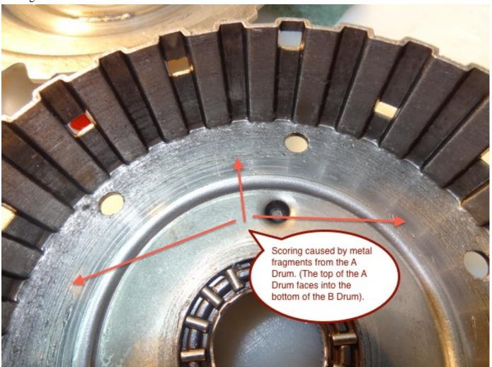
The scoring was at the interface where the top of the A drum fits into the B Drum and was where the material from the broken lip would have been located. The scoring appeared to have been caused by the material from the lip of the A Drum scouring the surface (this is a rotating drum). The scoring was not in an area where it affected operation of the B drum so, other than polishing the surface to remove sharp edges, the B Drum was reused.
