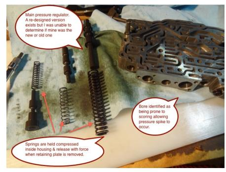
decided not to worry about it and re-assembled the valve body using the original pressure regulator.
