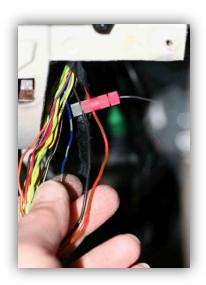
20. Next tap the **BROWN/RED** instrument cluster **left** connector wire with a *large Red/Slate* Posi-Tap. Then connect the **BROWN/RED** wire from the RealGauge harness.
