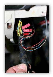
23. Pull the **right** side instrument cluster connector out and underneath the instrument cluster. Using a pointed pair of scissors, carefully snip the fabric electrical tape on the end near the connector. *Use care not to cut a wire!* Unravel the fabric tape and remove the foam or felt covering and set it aside. Also cut the end to unfasten and remove the inner black lacing tape wrap underneath the foam. Clean the sticky tape residue off of the wires using an alcohol pad.
