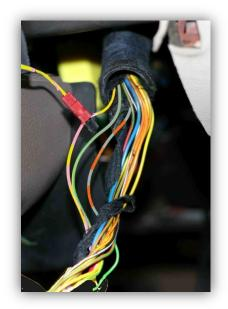
27. Next tap the **SLATE/GREEN** instrument cluster **right** connector wire with a *small Red/Black* Posi-Tap. Then connect the **SLATE/GREEN** wire from the RealGauge harness.
