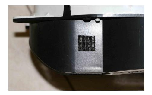
12. Install the RealGauge computer module on the Velcro with the label facing front. Align the left end with the curvature inflection point. The back end should be flush against the black plastic, and wedged under the white plastic protrusion.
