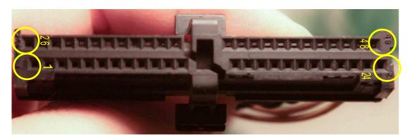
Sort through the instrument cluster **left** connector wires and separate out the **BLACK** (pin #26), **BROWN/RED** (pin # 25) and **SLATE/BLUE** (pin #10) wires from the rest of the bundle. (Note: The wires may have lengthwise color stripes instead of bands as in the photo).
