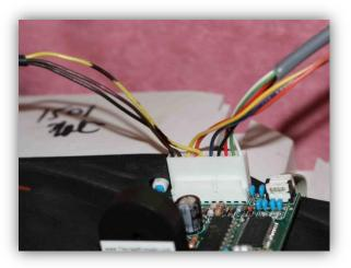
15. With the harness cables hanging on the right and left sides from the last step, replace the instrument cluster in the vehicle by tilting the bottom in place first. *Be sure the harness cables remain in front of the four mounting brackets. Do not* plug the two instrument cluster connectors back in at this time. Press down on the RealGauge module slightly, if necessary, to clear the dash opening while you rotate the upper part of the cluster into the opening.
