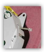
11. Place the instrument cluster with the top facing you. Using an alcohol pad, clean the black plastic surface above the gas gauge and above the tachometer area on top of the cluster and let it dry. Mount the 1" x 2" self-adhesive Velcro strip over the fuel gauge along the curvature inflection line, as shown below.
