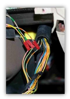
29. Use a tie wrap to strain relief the connections. Rewrap the lacing tape around the harness and then replace the foam or felt around the harness. Secure it with the original fabric tape, wrapping the ends with electrical tape. If the original foam is badly deteriorated, self-adhesive weather-strip foam from any hardware store can be substituted.
