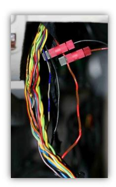
21. Next tap the **SLATE/BLUE** instrument cluster **left** connector wire with a *small Red/Black* Posi-Tap. Then connect the **SLATE/BLUE** wire from the RealGauge harness.
