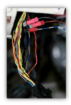
22. Use a tie wrap to strain relief the connections. Rewrap the lacing tape around the harness and then replace the foam or felt around the harness. Secure it with the original fabric tape, wrapping the ends with electrical tape. If the original foam or felt is badly deteriorated, self adhesive weather-strip foam from any hardware store can be substituted. The foam or felt is primarily used to prevent wire abrasions and rattles.
