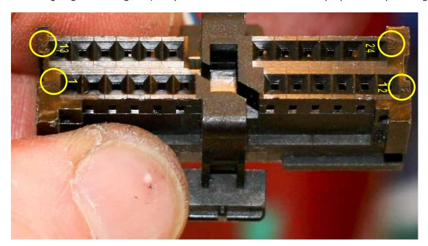
25. Sort through the instrument cluster **right** connector wires and separate out the **PINK/YELLOW** (pin #3) (may also be **PURPLE-YELLOW**), **SLATE/GREEN** (pin # 4) and **ORANGE/SLATE** wire on **pin # 19** or **pin # 21 (on very early cars)** of the instrument cluster **right** connector (you need to check this pin number because there may be more than one **ORANGE/SLATE** wire) from the rest of the bundle.
