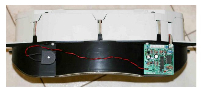
14. Plug the 10-position white connector from the RealGauge wiring harness into the computer module as shown. Make sure the stops on each corner of the 10-position connector face toward the front of the instrument cluster. Seat the connector fully. Separate the shorter three-wire cable to the right, and the longer three-wire cable to the left. (Note: The four-wire cable with a gray jacket shown in the photo is not used on XJ/X308 models).
