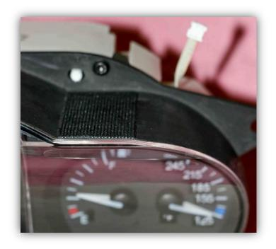
Mount the 3/4" x 3/4" self-adhesive Velcro strip over the tachometer approximately as shown below.
