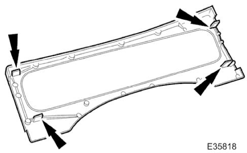
4. Using a thin plastic lever, carefully release the four centre veneer panel dowels from fascia clips.
