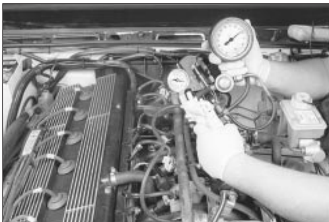
3.9 Check fuel pressure without vacuum applied to the fuel pressure regulator, then with vacuum applied; fuel pressure should DECREASE as vacuum INCREASES
