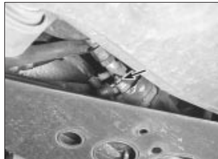
3.3a Remove the rubber boot from the fuel pump electrical connector and check for voltage while an assistant turns the ignition key (1989 model shown)
