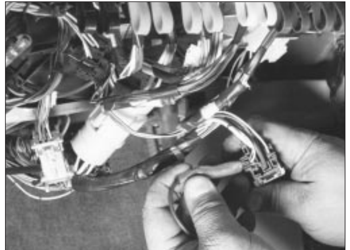
3.3b Checking for battery voltage to the main relay (1989 model)
