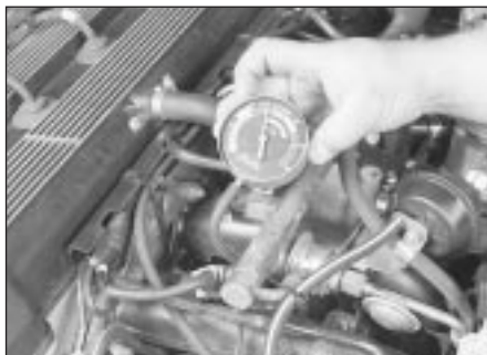
3.14 Connect a vacuum gauge to the vacuum line leading to the fuel pressure regulator and check the vacuum source
