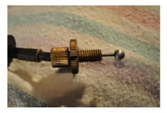
Check and ensure the choke cable is fully extended, that means pushed all the way in at the inner control, and the "fast idle" cam is NOT in contact with the "fast idle" setscrew.
