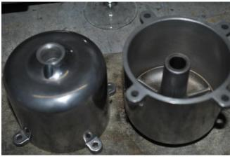
Now check the piston outer circumference, paying particular attention to the 2 grooves. Use a nylon brush with kero to clean this up as good as the bell chamber.
