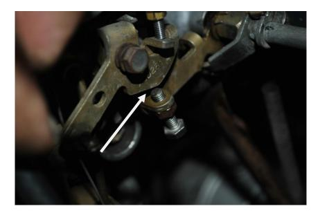
Note the "Z" clamps securing the throttle rod joining the 2 carbies (the rod closest to the manifold, as the outer one is the choke shaft joiner, if fitted). Loosen the small bolts (just loosen will do), enough so that the front carby shaft moves without the rear carby shaft moving at all. You need both carbies to be separated to get the adjustments correct.
