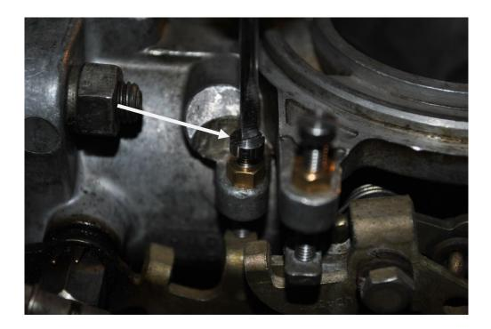
These 2 adjustments are a "base line" setting I have found to work well for initial starting in 90% of cases. Some idle a tad slow, so rotate EACH idle screw a further ½ turn. They MUST be rotated equally to maintain a basic balance. Fine tuning of the balance will be done shortly.
