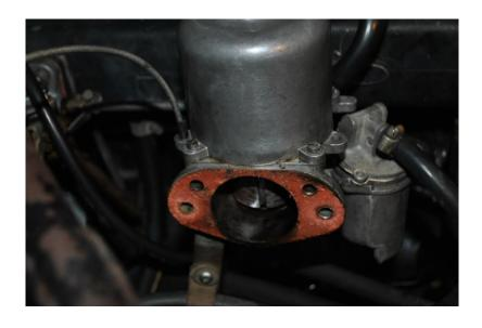
Ensure the throttle cable has "some" slack in it, coz if it is too tight the whole next procedure is a total waste of time. I generally disconnect it totally and sort the refitting after the work is done.
