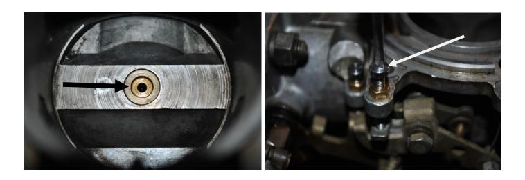
Loosen the locknuts on the idle speed screw, and rotate it anti-clockwise until clear of the stop arm. Rotate it back down until it JUST CONTACTS the stop arm, now go down ONE rotation. Now do the same with the other carby.
