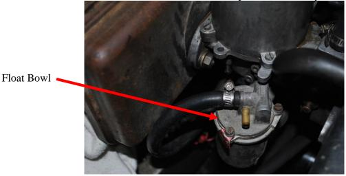
Invert the lid (float upward) and place your mouth over the fuel inlet pipe and SUCK, and ensure you CANNOT suck air. If air is sucked, FAIL. Once vacuum is achieved, turn the lid over (float downward) and blow through that pipe, and carefully raise the float, thus closing the needle, and ensure your "puff" is closed off.
