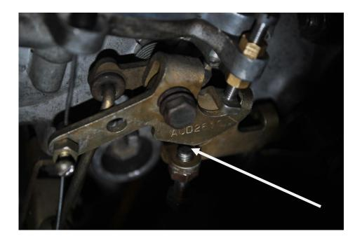
Some fine tuning may be needed as things settle, and the 2 separated carbies situation is only required if idle speed is being played with. The mixture screws only affect the related carby.
