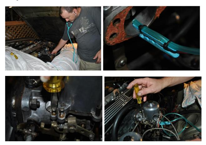
Or source a stethoscope from a nurse and some oxygen tube to lengthen it, and attach to the carby throat with a cloths peg.
