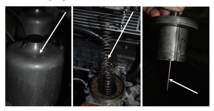
Note: All parts removed must be kept separate so that they can be re-installed into their correct carby. Multiple plastic ice-cream containers are useful.
