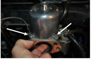
If it is OK, remove the chamber, fill the centre tube of the piston with ATF (trans fluid), to about ½" from the top. I used a 2ml syringe with about 50mm of vacuum tube on the end, and added 2 Syringes of fluid.
