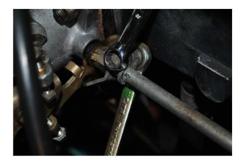
Reconnect the throttle cable ENSURING that NO throttle linkage movement is occurring when sliding the clevis pin through the connector. Some cable slack is needed, and I usually allow 2mm or so, and it really is a "feel thing".
