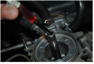
slide the spring over, and refit and secure the chamber. Check that "smoothness" again.
