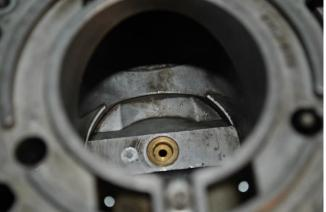
While I had Bell chambers off it was a good time to replace a miss-matched set of idle and mixture screws. Idle screws are 4 BA x  $^{3}4$ " SS cheese head, Mixture screws are 4 BA x 1" SS cheese head. Lock nuts are 4 BA Brass nuts. You can try to source these locally but in Brisbane I found only two 4 BA bolts and they were the wrong length, 5/8". SU Midel in Sydney had them at a premium price.
