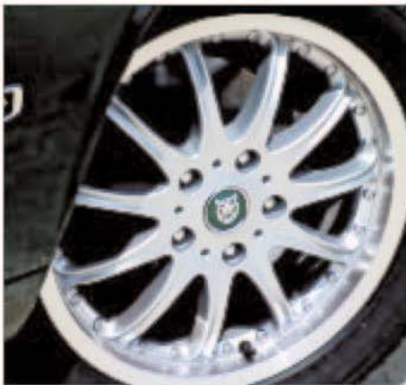
Seventeen-inch alloys look smart and have been properly set up with the correct spacers and hub fittings to suit the XJ-S
