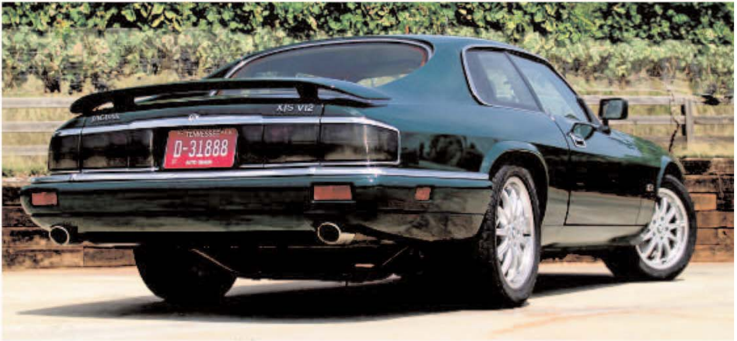
From the rear you can just make out the specially developed sports exhaust – a complete kit that boosts power by 20hp
