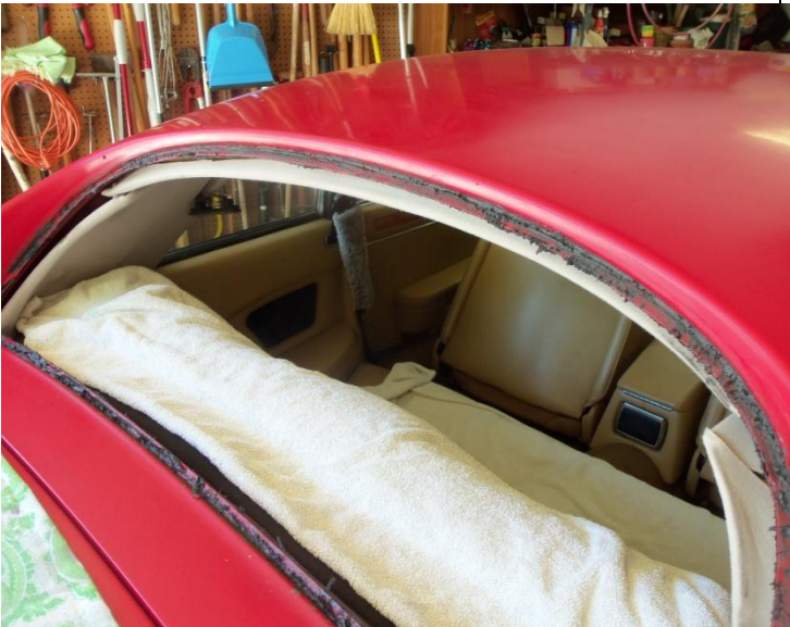
Remove the gasket and set it aside where it will not get anything messy from the sealant on it.
