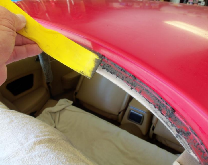
The yellow putty knife worked quite well in scraping off most of the sealant, as can be seen ...
