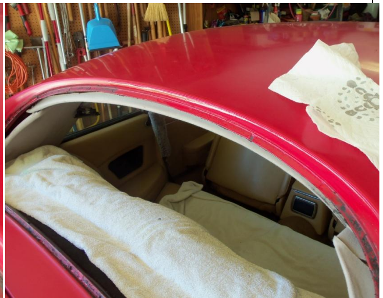
... works quite well is wiping off the remaining sealant.
