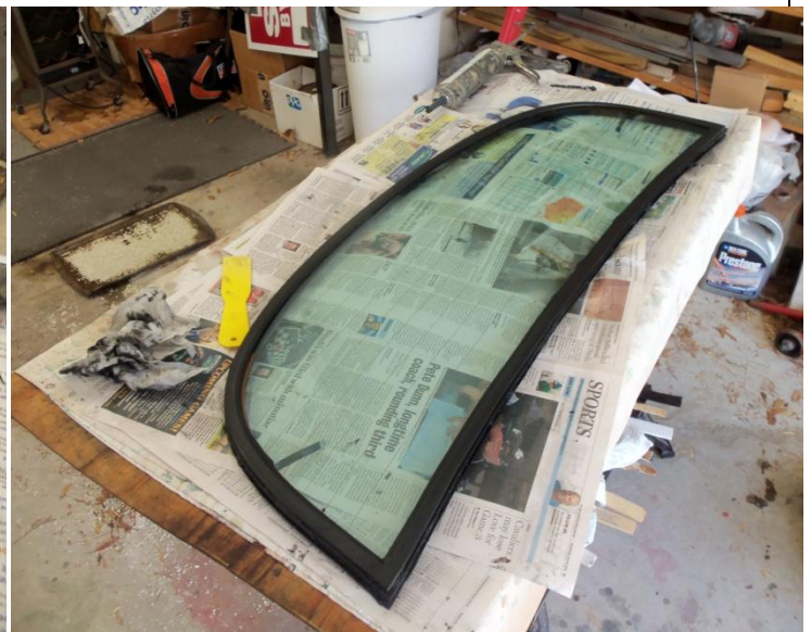
The rear glass is fully in the gasket and ready for the next step – installing the chrome trim.
