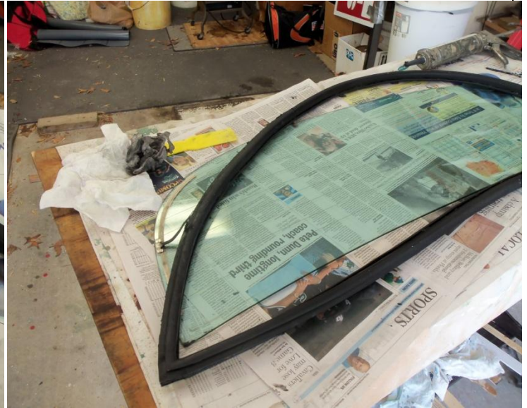
The gasket now has sealant around the entire inside groove which will receive the glass.
