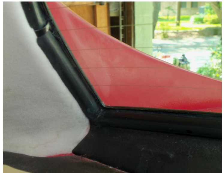
Closer view from inside, shows the headliner pieces tucked into the gasket lip as intended to be.
