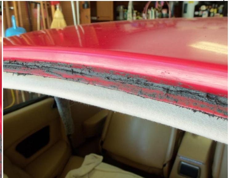
This (and the previous photo) shows the sealant which remained on the pinch-weld after removing the gasket.
