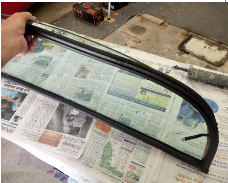
Start by setting the glass in the bottom of the gasket, then with the glass vertical (or mostly vertical, however you have to tilt it to work with it), then push the gasket onto the glass so the glass is snugly in the gasket.
