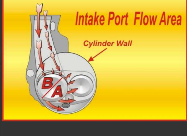
When the valve is lifted to about the 0.450-0.500 range the air, although with streamlines far less tidy than shown here, enters the cylinder about like this. The bulk of the air passes out of the port and into the cylinder through the half of the valve labeled `A'.
