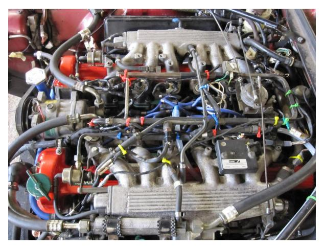
The pipe concerned is the grey steel one that runs across the middle of the engine from the top centre of each manifold, and then the leg of the T shape runs forwards (leftwards in the photo) and downwards behind the manifold at the bottom of the photo. It has a yellow cable tie on it (the leftmost yellow tie in the photo) and a blue cable tie on it in its centre between the manifolds.
