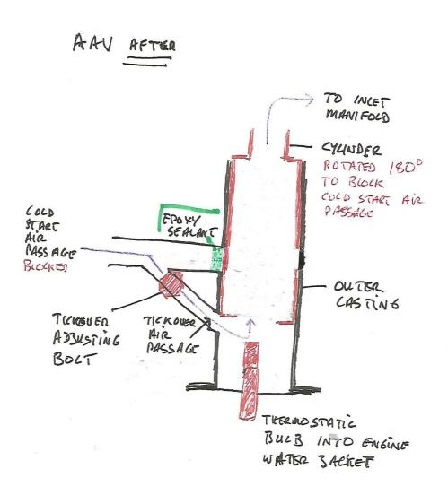
As the diagram shows, the AAV casing has been emptied of its moving parts except for the slow running (tickover) adjustment function. The AAV was then reinstalled on the engine just as before. There is no need to touch the thermostatic bulb.
