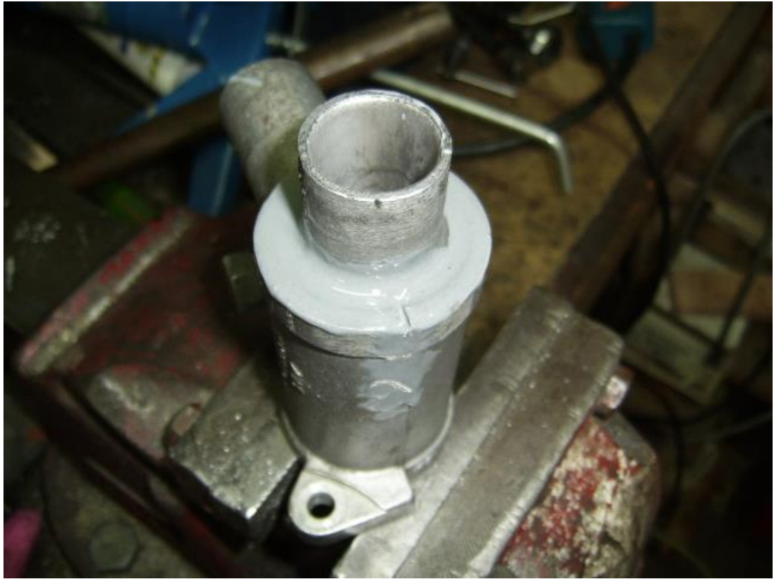
Completed unit with JB weld in place.
