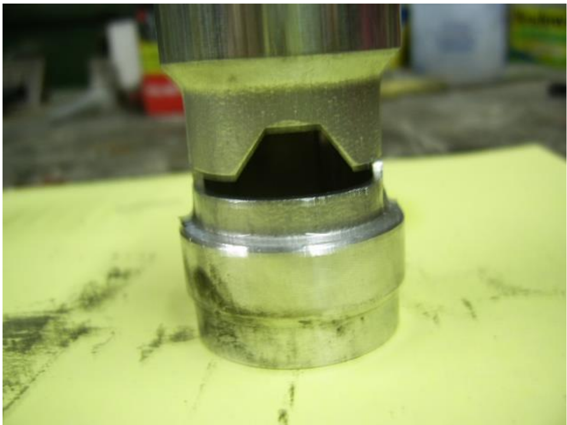
Tophat showing the cut outs that control cold idle.
