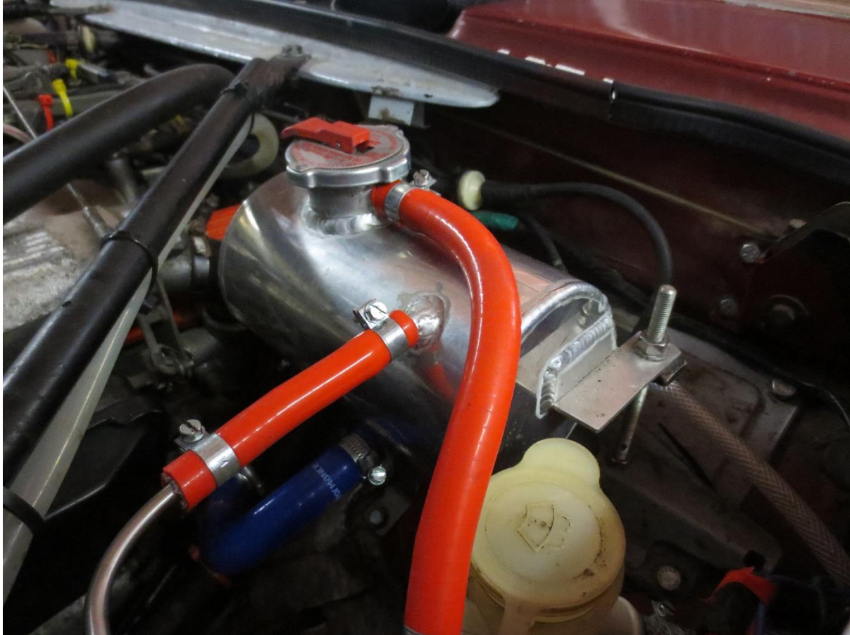
FIG 7 New expansion tank by the bulkhead
