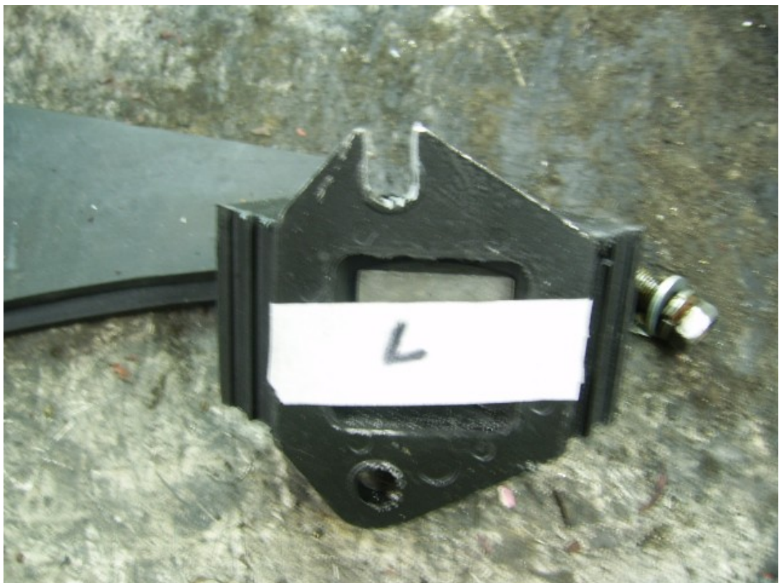
LH mount showing the slot and the offset for fitment.
