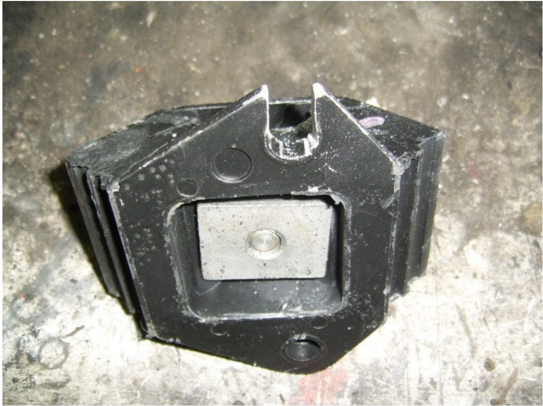
RH mount showing the slot. Also note the offset for handed refitment.
