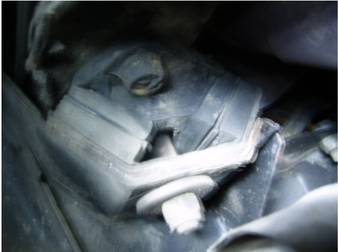
LH V mount as fitted to the car, with separation clearly visible
