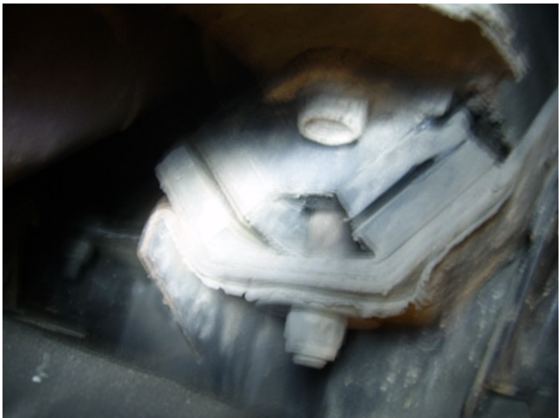
RH V mount in situ showing separation
