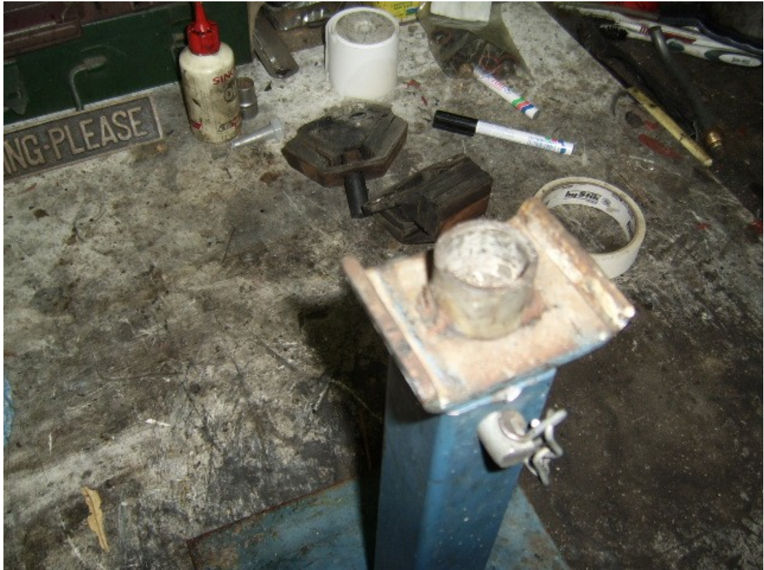
My jackstand showing that pipe welded to the top face.
