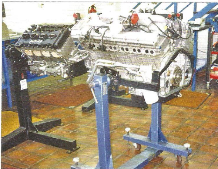
HB Cosworth 'Jaguar' 3.5 V8 and the new Eng's designed 4 valves per cylinder 6.4-litre V12 engine, for road use. This 6.4 litre V12 fitted to a Jaguar XJR-S saloon, and the performance tests are shown above.
