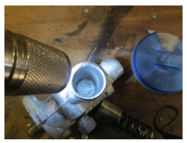
An important point to understand is that blocking this air passage does NOT block the function of the slow running adjustment screw. The air passage for the tickover adjustment has a separate route through the casting. In diagrammatic form, this is what has been done:
