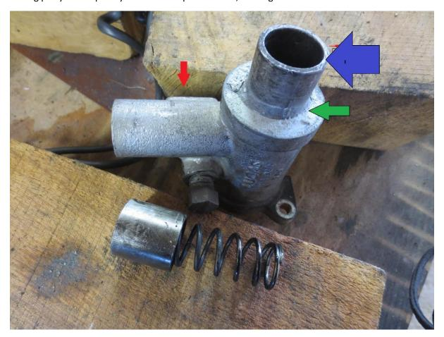
cylinder, the **green arrow** indicates where the cylinder has been released from the outer casing and turned 180 degrees to close the air passage and then resealed; the **red arrow** indicates the air entry tube from the air filter box. The original air passage opening is at the cylinder end of this air passage. The piston has been removed from the unit as is obvious. The following photo shows the air passage at the cylinder end completely sealed with epoxy putty.
