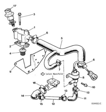
In the diagram, the air inlet is at the side of the solenoid and the outlet to the manifold is at the bottom of the unit. This solenoid flows enough air to enable the V12 to tickover at about 800 RPM when stone cold at an ambient temperature of 0 degrees C (32 F). The photo below shows the unit:
