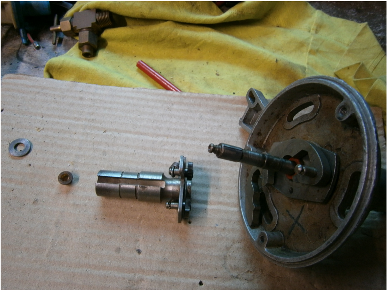
Here it is. That “Split Collar” is the thing on the far left. The “nipple” it sits over is clearly visible on the top of the Inner Shaft.
