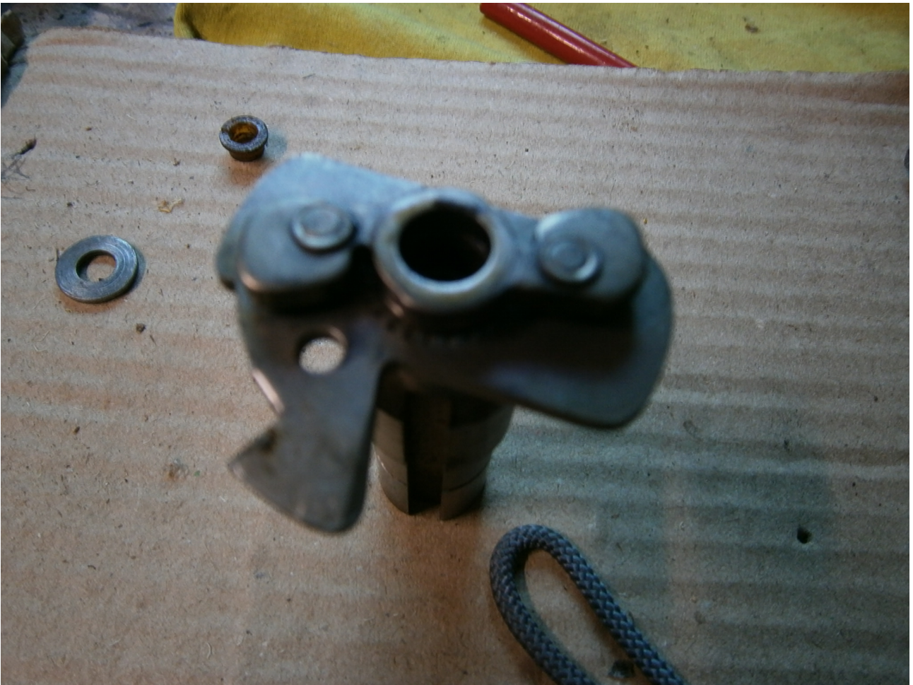
Underside of that "Outer Shaft" showing the "knobs" that engage the weights. That washer is NOTHING to do with this, just me being slack and not clearing the work space.
