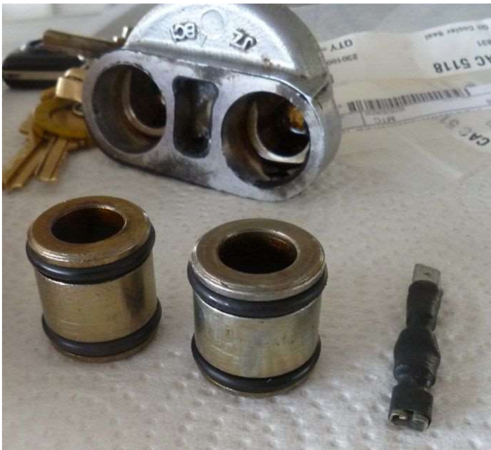
Figure 3: Detail of metal sealing collars and “O” rings (thanks to Lawrence for the pic.)
