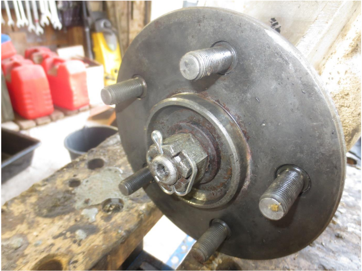
Photo 24: outer thick washer, nut and split pin fitted.
