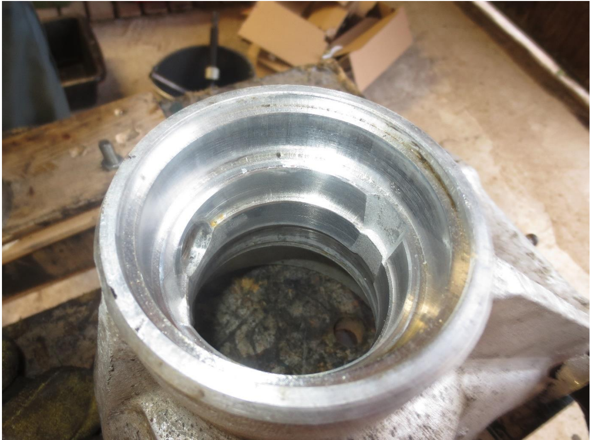
Photo 14: the empty hub carrier showing the indents that allow the outer races fitted to it to be driven out.
