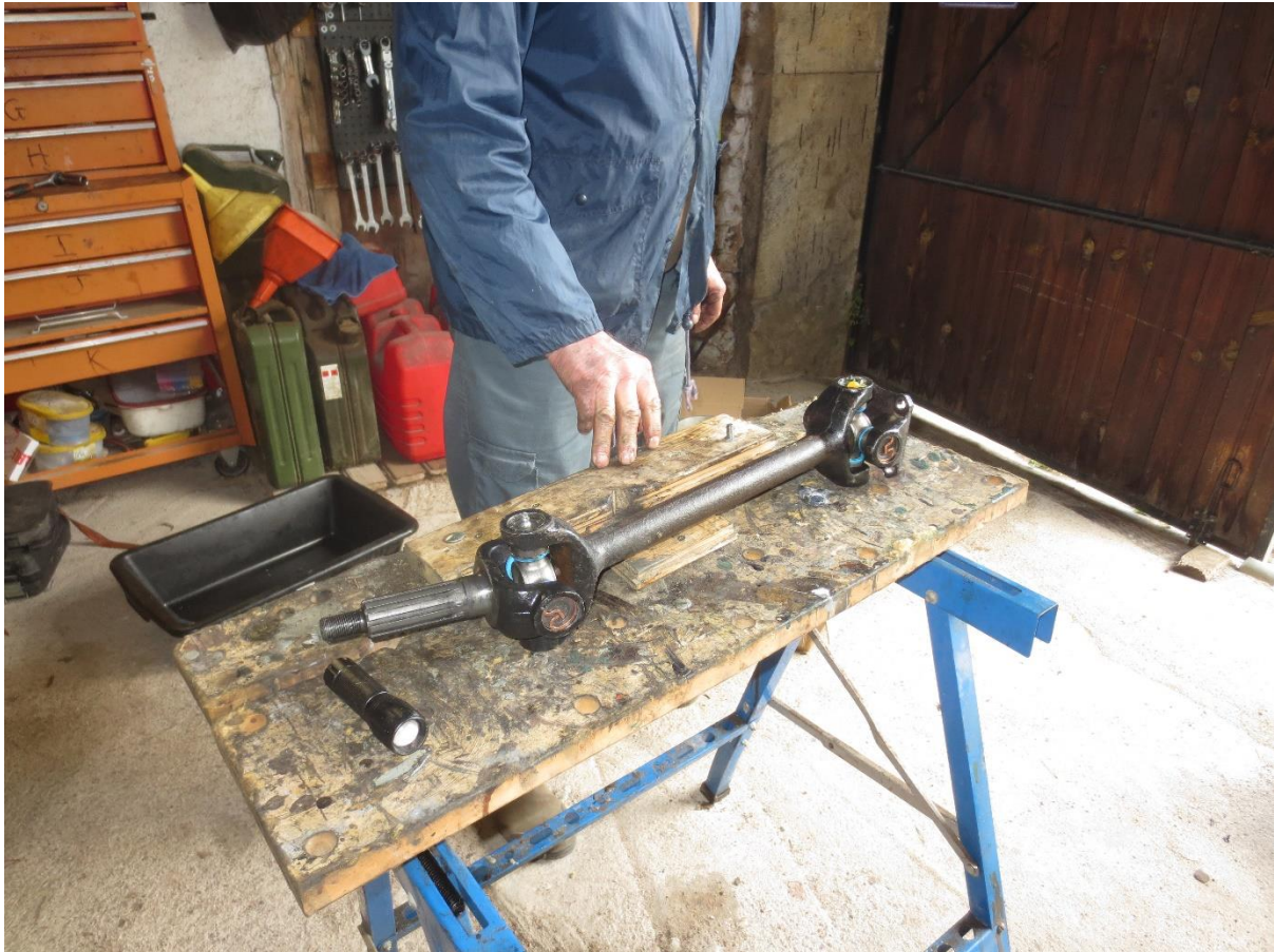
Photo 12: the clean driveshaft with derusted splines and shiny new UJs, ready to be refitted to the hub.
