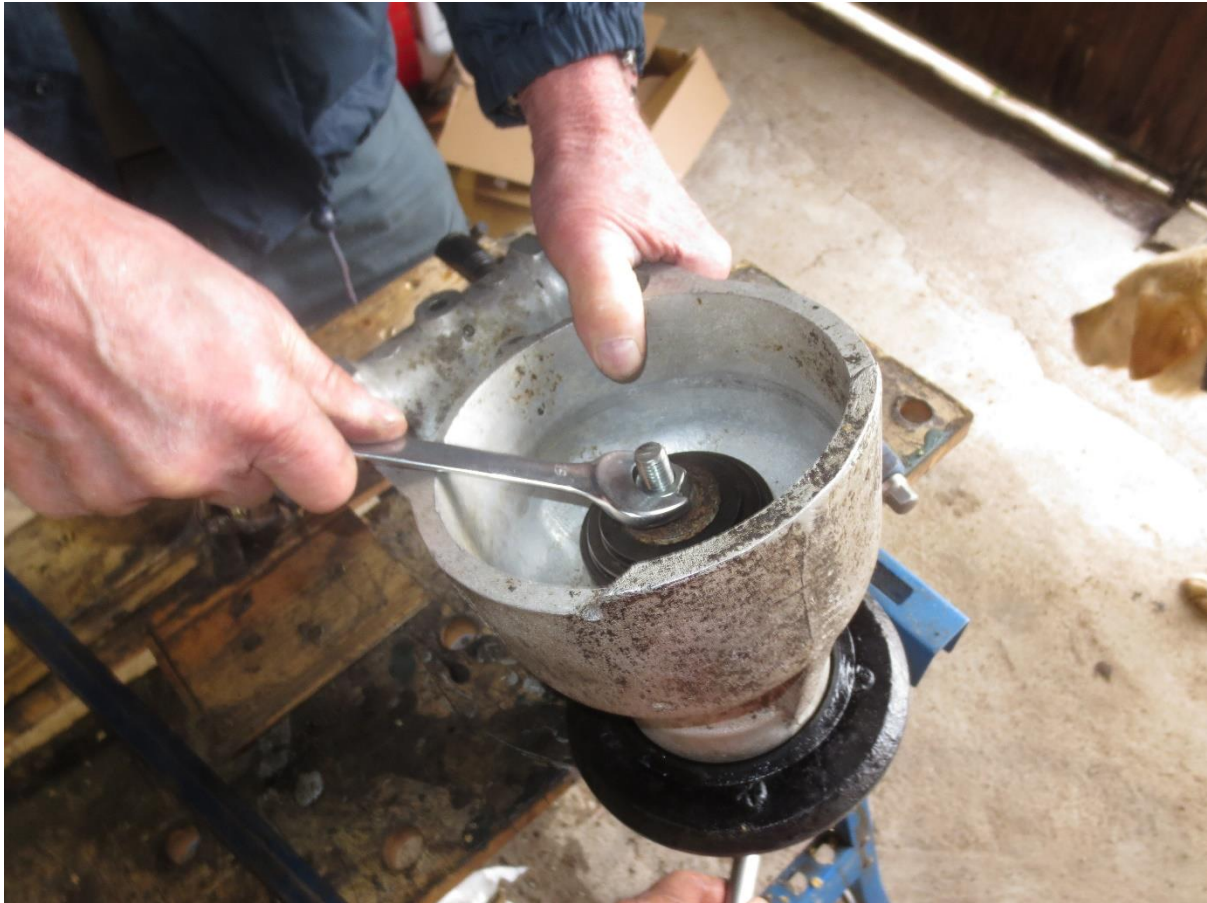
Photo 20: winding the inner bearing race over the hub tube.
