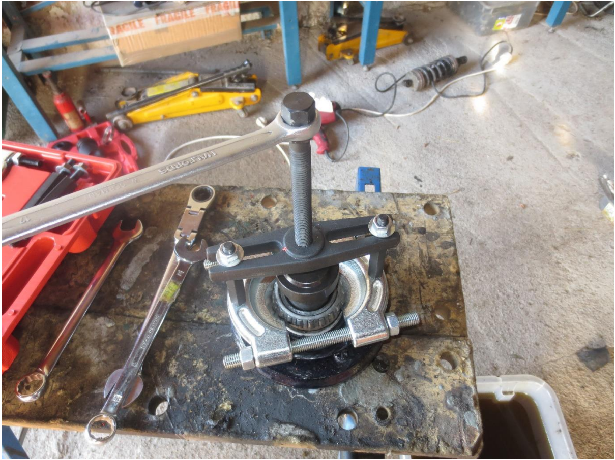
Photo 13: the bearing puller kit pulling the old outer hub bearing inner race from the hub.
