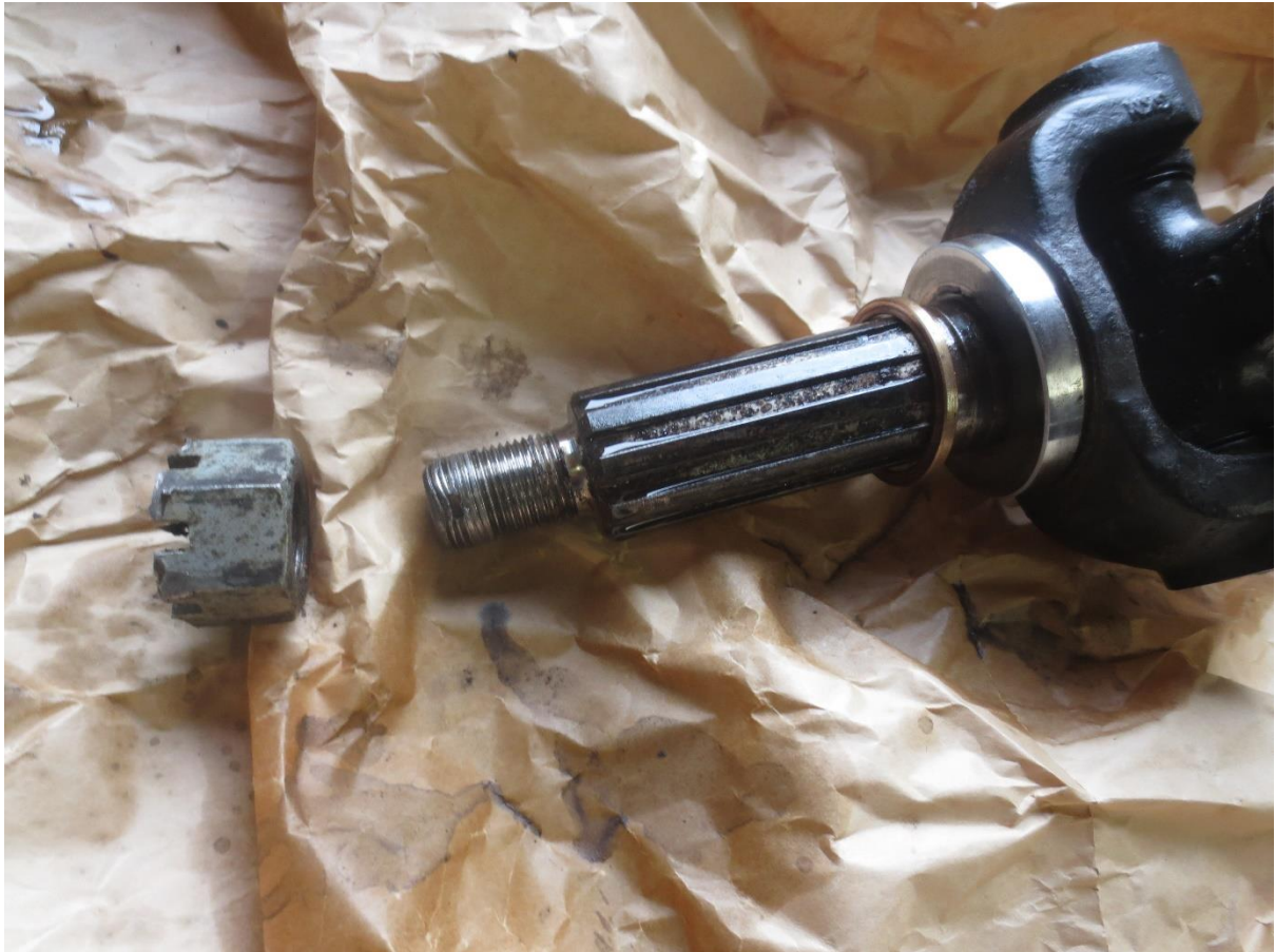
Photo 3: the male splined end of the driveshaft that fits into the female splines of the hub, and thus transmits drive to the hub and road wheels. Note the two spacers on it against the UJ yoke. These are important and must be carefully retained.
