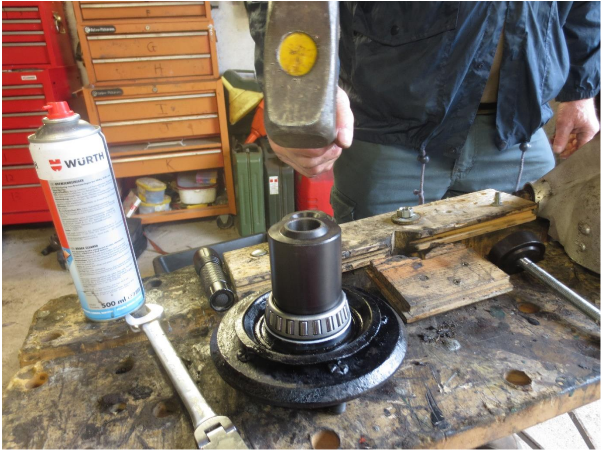
Photo 18: driving the new outer bearing inner race onto the hub. Next the hub is fitted into the hub carrier and the inner bearing's inner race placed in position. The inner race cannot be fitted to the hub tube by hand pressure, it too has to be wound in place. Photos 19 and 20 show the stages required:
