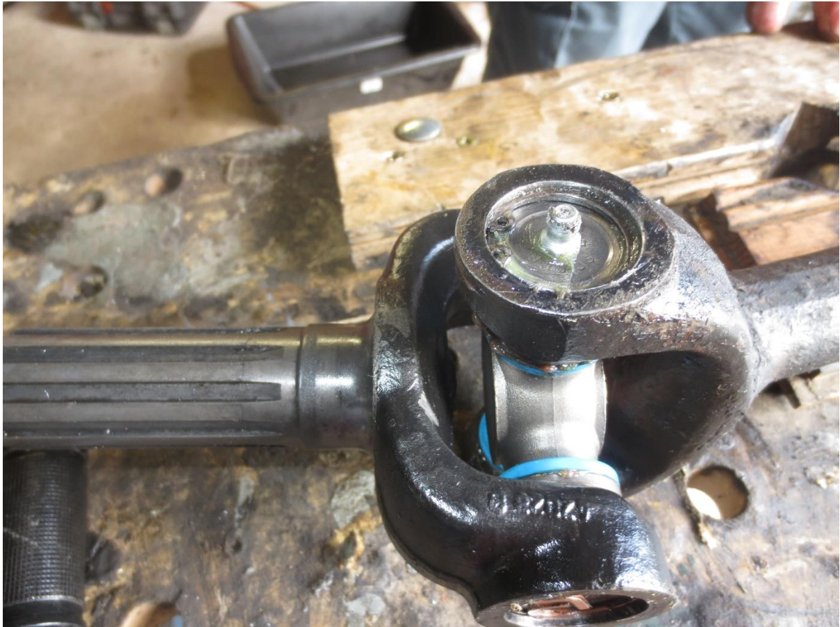
Photo 10: the new UJ fitted into the driveshaft yokes.
