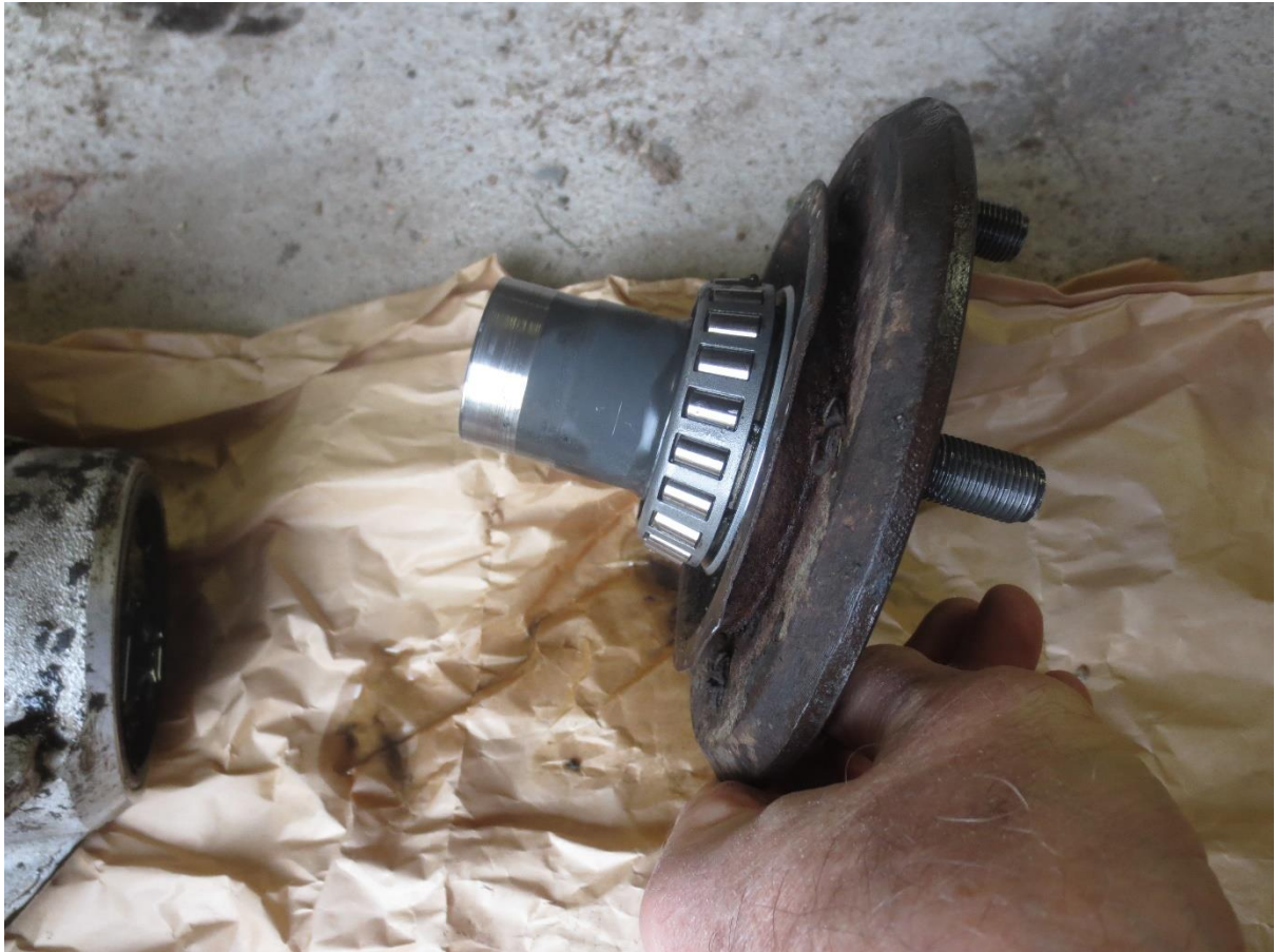
Photo 2: hub with outer bearing's inner race still in place. The inside of the hub tube is machined with female splines
