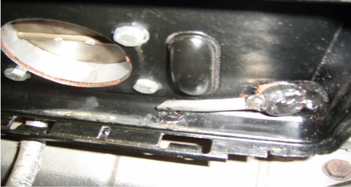
Inside the LH air filter showing the distributor cap vent pipe. A little “rough” looking, but was tidied up later, but forgot to re-snap it.
