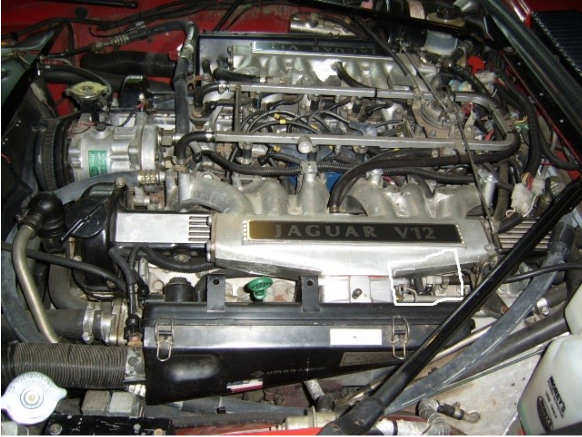
Figure 1 Just showing 1 cold start solenoid inside the White square
