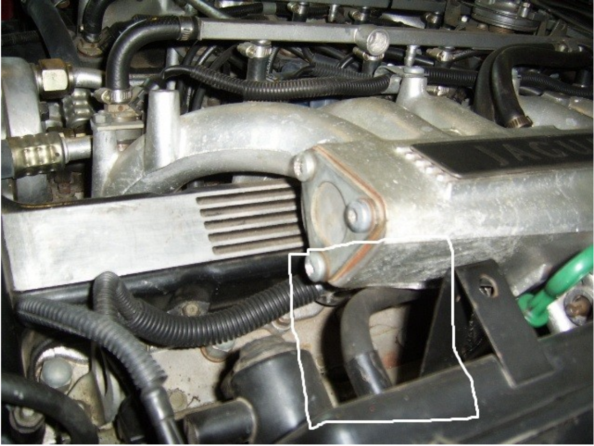
Figure 2 Solenoid air intake.
