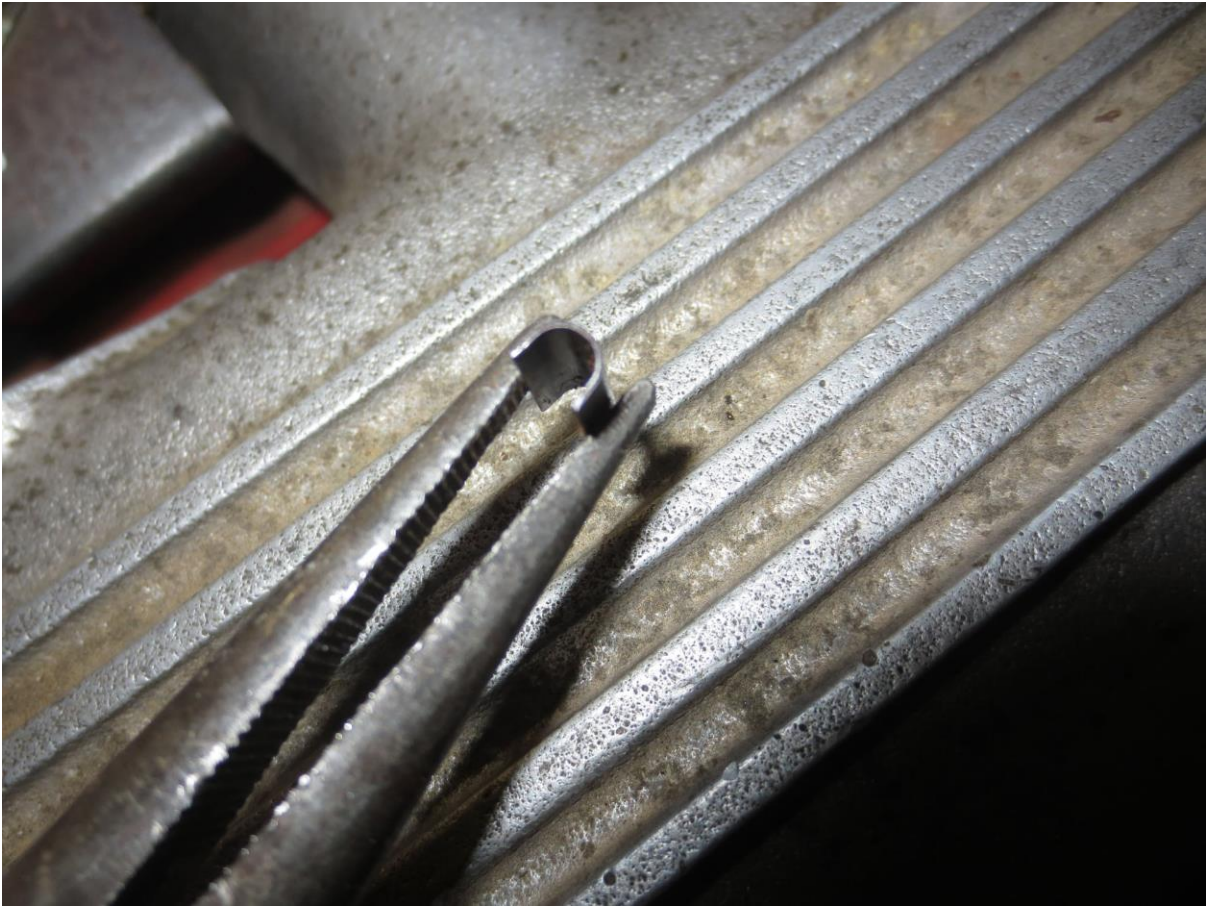
U clip in pliers ready to be replaced
