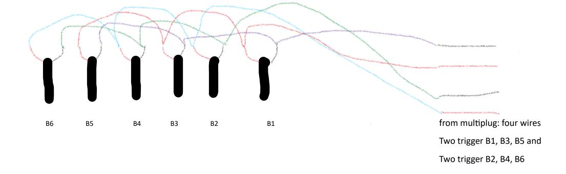
The plan I have is to use silicone covered wire running inside a thin silicone tube as an outer. The only joins in the wires would be at the crimped connectors, providing the wire, which will have to be quite thin gauge, will carry the current.
