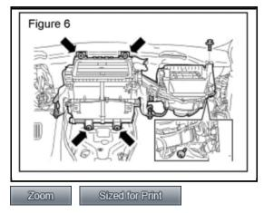
5. Install the heater and evaporator core housing (Figure 6): ^Tighten the bolt to 7 Nm +/- 1.1 Nm (5 lbf ft +/- 0.8 lbf ft).
