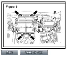
2. Release the heater and evaporator core housing for access to the drain tube (Figure 1): ^Move the carpet for access
