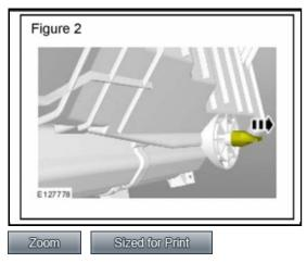
3. Remove and discard the drain tube from the rear of the heater unit. (Figure 2)
