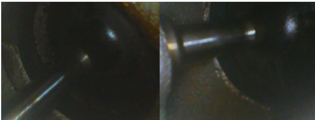
Figure 12: AAA engine borescope inspection, pre-test (left) and post-test (right).
