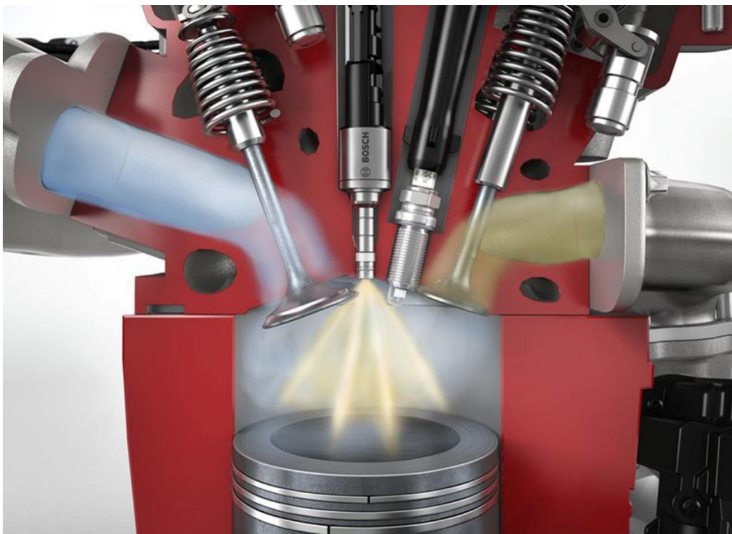
Figure 5: Gasoline direct injection engine illustration fuel spray directly into combustion chamber. Image Source: Bosch
