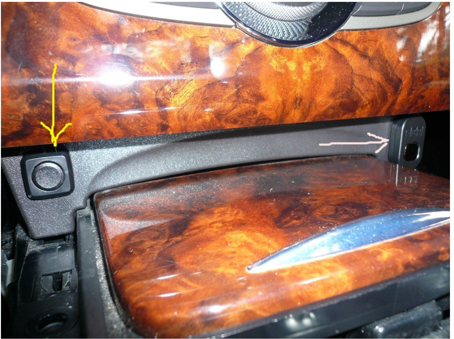
Run the wire back to the respective box. Yellow arrow is the switch and the other is the wire. Side view with side of console removed.
