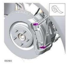
CAUTION: Removal of the clips is a delicate procedure, damage will occur if any force is used.
