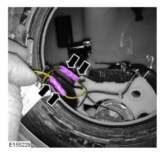
17. CAUTION: After crimping the connection, perform a gentle pull test to make sure that a sufficiently strong connection has been created. If required, remove and replace the splice.
