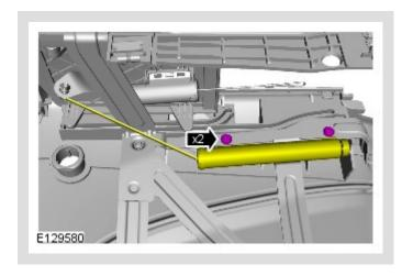
Release the air damper unit from the trim panel.
