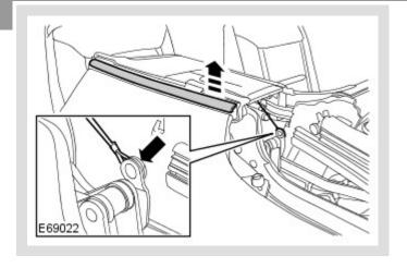
Carefully remove the outer waist seal.
