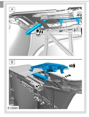
Remove the rear quarter trim sliding panel complete with both air damper units
