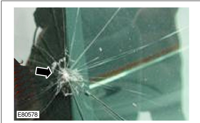
11. High impact resulting in many cracks.
