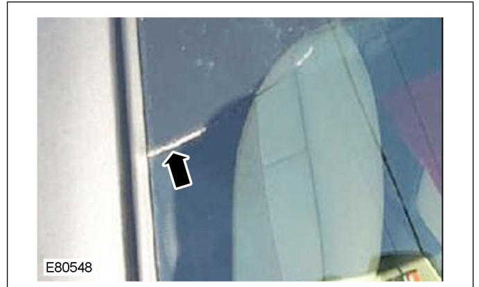
14. Crack along A-pillar.
