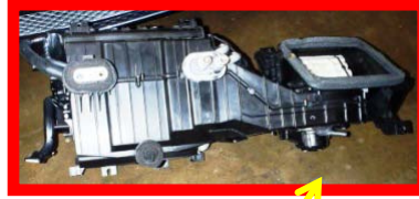
Water leaks from the Fan Motor that is located under the glove compartment
