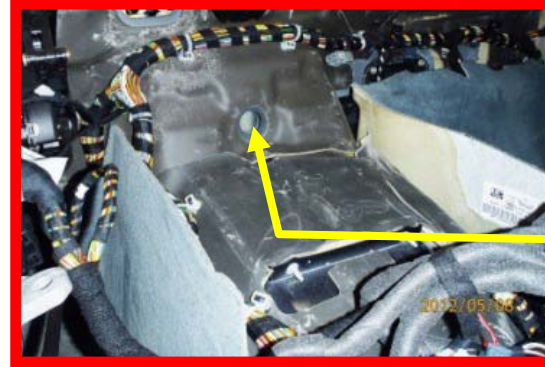
Drain Hole Through Firewall exits just above transmission housing
