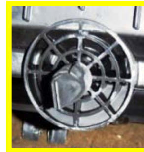
Duck bill Hose with the sealing material removed. (Duck Bill Design to prevent insects coming into the car?)
