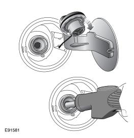
To remove the filler cap, turn it counterclockwise approximately a ¼ turn, until a slight resistance is met. Continue turning to release it. Remove the cap from the filler neck.
