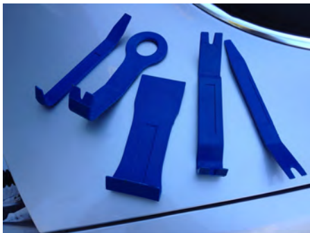
Plastic Interior Panel Removal Tools from Harbor Freight used to assist in removing the plastic antenna cover from outside the vehicle.
