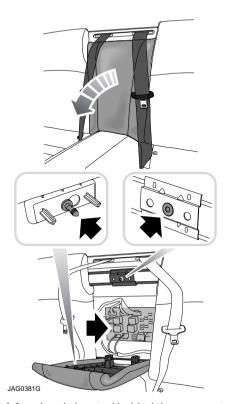
A fuse box is located behind the rear seat centre section.
