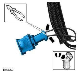
**14.** Using a suitable tool, remove 5mm of insulation from the end of each wire.
