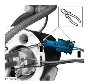
**8.** Using a suitable tool, remove 5mm of insulation from the end of each wire.
