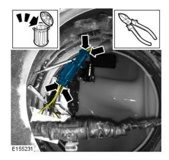
18. CAUTION: After crimping the connection, perform a gentle pull test to make sure that a sufficiently strong connection has been created. If required, remove and replace the splice.
