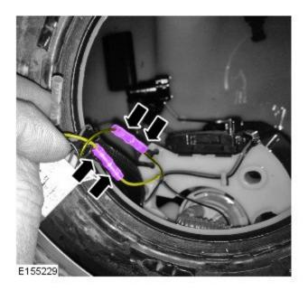
19. CAUTION: After crimping the connection, perform a gentle pull test to make sure that a sufficiently strong connection has been created. If required, remove and replace the splice.
