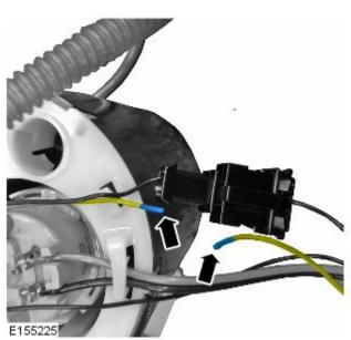
9. CAUTION: After crimping the connection, perform a gentle pull test to make sure that a sufficiently strong connection has been created. If required, remove and replace the splice.
