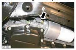
5. Disconnect the engine oil pressure (EOP) sensor electrical connector.
