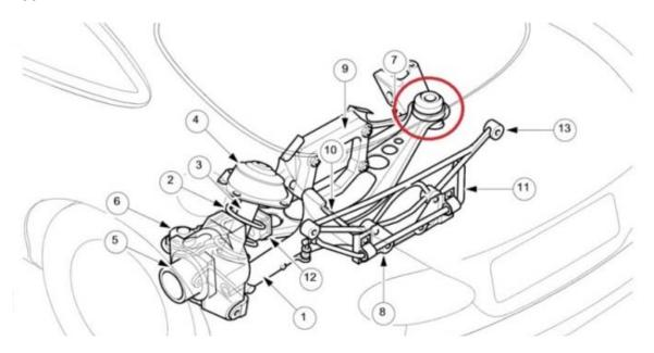
The XK8 rear suspension design shown in the line drawing above reduces the natural tendency of the car to squat under acceleration. Like the front end, the XK8 rear suspension utilizes a control-arm design, with the coil spring and damper combined into a single unit. The spring is seated directly on the cast-iron transverse lower wishbone, not the damper, which reduces friction for better ride comfort and noise isolation. The half-shafts serve as the upper suspension links.
