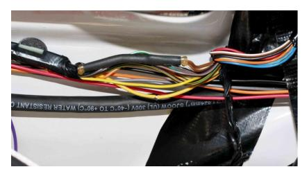
**Step 16:** Pull the violet wire from the relay/timer wire assembly back from the speaker area to the central area of the harness discussed in step 14 above. Solder the CATHODE (white striped side) of a 1N4001 diode to the LEFT side of the cut yellow wire AND to the violet wire. Slide on heat shrink tubing. Solder the ANODE of the diode the RIGHT side of the yellow wire. This is illustrated below photos:
