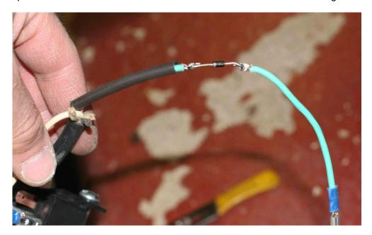
**Step 36:** Fold the diode back over the black line code cable jacket and tape it in place with electrical tape. This will provide protection and strain relief for the diode.
