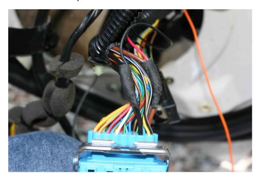
**Step 12:** Continuing with DD10, the blue connector, solder tap the yellow wire (DD10, terminal 5) to the orange wire from the relay/timer wire assembly. Double check this is the SOLID yellow wire on terminal 5, and not a yellow wire with a colored stripe. See below.
