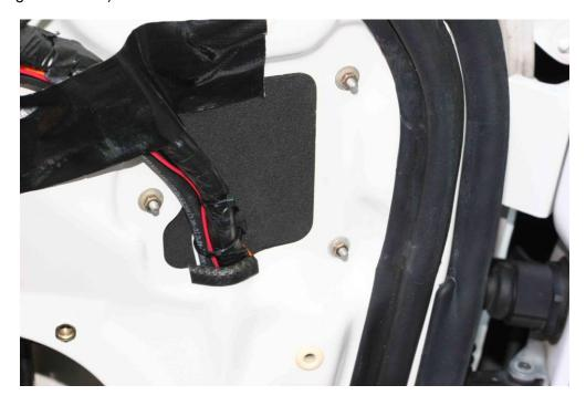
**Step 6:** Carefully extract the driver door module from the inside of the door cavity with the attached cables through the speaker opening. Make sure you do not lose the foam gasket inside the door.
