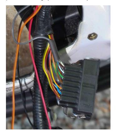
**Step 14:**. Re-tape both of the Driver Door Module connector harnesses with vinyl electrical tape up to near the connector bodies.
