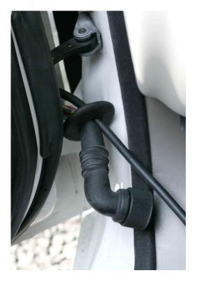
**Step 22:** Neatly dress the cable to the boot with two black tie wraps as show below:
