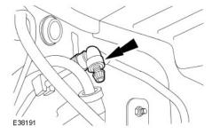
To comply with Standard Federal Testing Procedures (SFTP) a test port is provided in the evaporative emission canisters to purge valve resonator line to enable leak test diagnosis of the fuel system.
