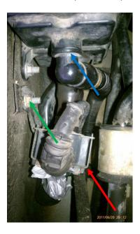
Unplug the CCV (Sqeeze the connector after you slide the boot back)
