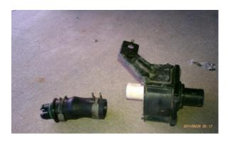
Check the seal that goes in to the canister. (Green seal) While you have the little hose off you should replace it. Jag mechanics point to this hose as the usual problem, because it dry rots and splits. You can buy hose for this at Autozone or other auto joints. You can also order the OEM from Terry's Jaguar (<a href="http://www.terrysjag.com/">http://www.terrysjag.com/</a>) (800-851-9438)
