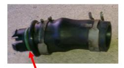
If these are ok, you can follow the top hose to the other side. It curves down and goes into the bottom of the 2<sup>nd</sup> canister (Blue Arrow Below). This side is not as easy. Here is where the CCV Canister Close Valve is located. (Red Arrow) The Canister close valve is held on by the hose and the bolt. (Green Arrow)
