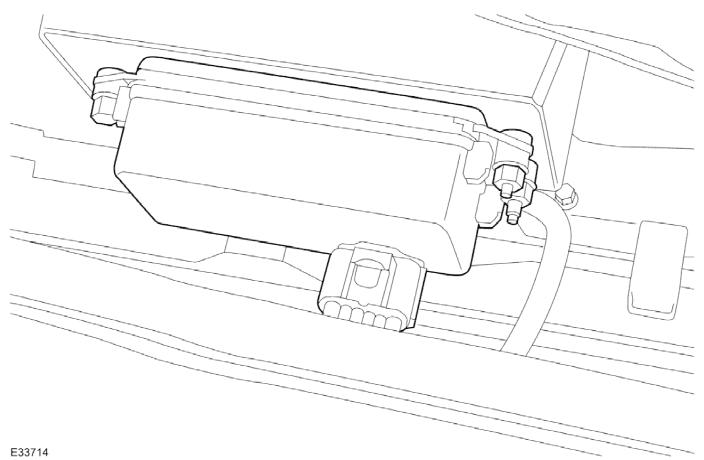
An adaptive speed control, control module (adaptive SCCM) incorporating a radar sensor and yaw rate sensor provides system control functions. The SCCM is installed in a mounting bracket located in a cut-out in the body front upper crossmember.
